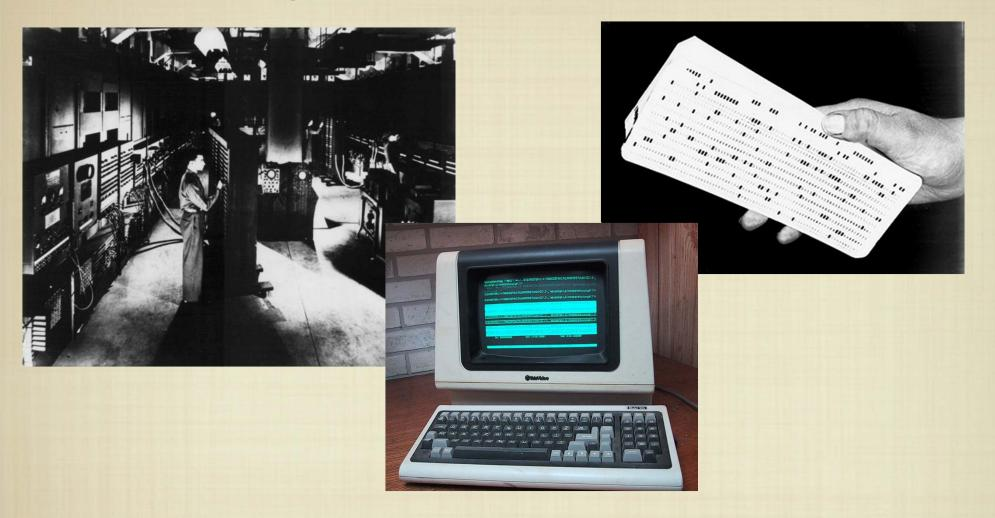
Computer programs were first manually loaded and executed on mainframes. "Terminals" became popular in the 1970s as CRTs became inexpensive.
